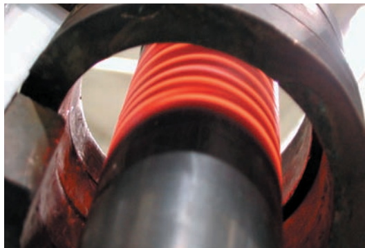
Fig. 1 — Multiple stripes appear due to a striping phenomenon. (Note that the induction coil has only four turns.)
