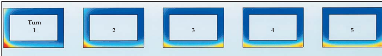
Fig. 2 — Current density distribution within coil turns in a multiturn induction coil. (Turn numbers correspond to those in Fig. 1.)
