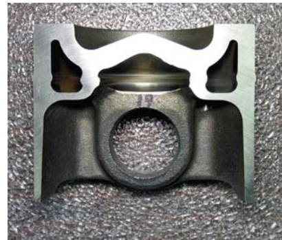
Fig. 3. Spinduction™ produces consistently flawless welds at very low rotational velocities with minimum or no flash projection.
