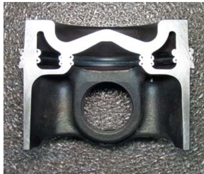
Fig. 2. Cross-section of a friction-welded piston
