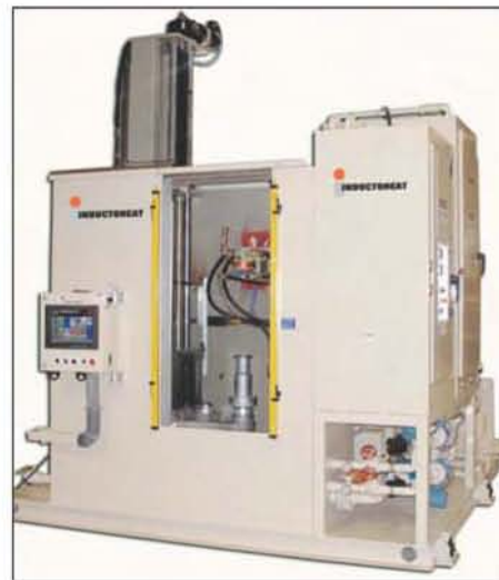
Fig. 7 — Inductoheat's single-coil dual frequency system comprises medium-frequency (10 kHz) and high-frequency (120 to 400 kHz) modules working simultaneously or in any sequence desirable to optimize properties of the heat-treated gears; total power exceeds 1,200 kW.
