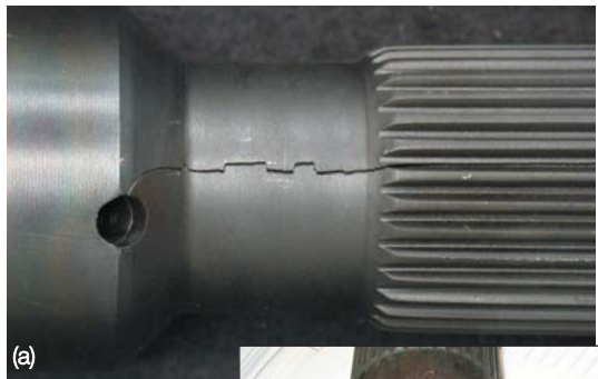
Fig. 1 — Cracks initiated in proximity to transverse hole (a) and longitudinal hole (b).
