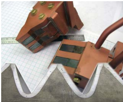
Fig. 3 — In tooth-by-tooth hardening, inductors can be designed to selectively harden specific areas of gear teeth where metallurgical changes are required (e.g., root, fillet and/or flank of the tooth) producing a fine-grain martensitic layer with minimum shape distortion. The remainder of the part is unaffected by the induction process maintaining its toughness and ductility.
