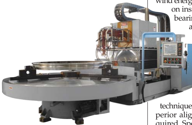
Fig. 4 — Induction gear-hardening machine for a large bearing ring for a wind-turbine generator with teeth located on the inside diameter of the ring. The bearing ring OD can be as large as 140 in. (3,500 mm). The required case depth is 2.5 to 3.5 mm, the z-axis scan height (tooth width) is 13.75 in. (350 mm), and the maximum weight exceeds 11,000 lb (5,000 kg).
