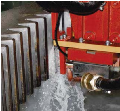
Fig. 2 — Tooth-by-tooth induction hardening can be applied to external and internal large gears and pinions requiring the inductor to be symmetrically located between two flanks of adjacent teeth.
