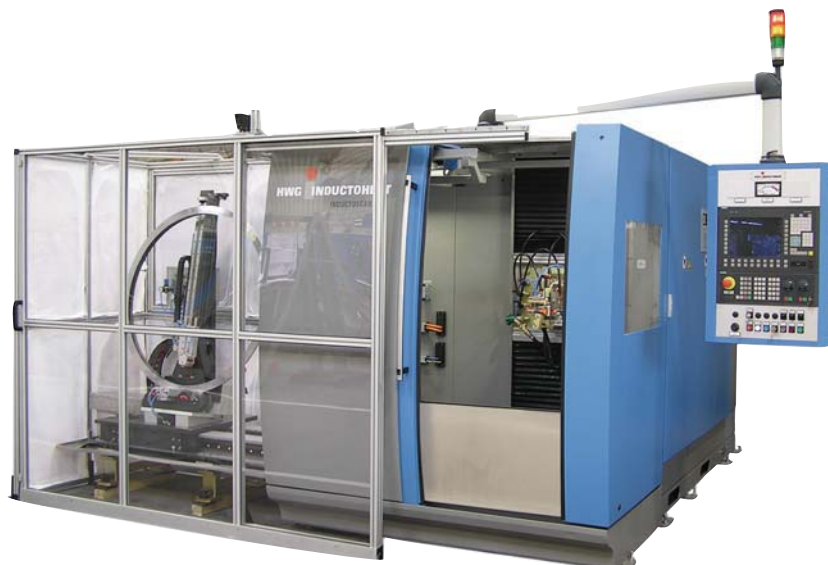
Fig. 5 — InductoScan base compact machine for bearing ring induction scan hardening. Rings are loaded into position by crane. Scan hardening is managed using Siemens 840D control.
