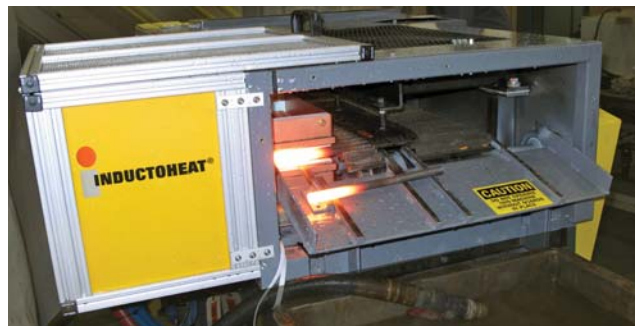
Figure 2. Induction bar-end heating using channel (slot or skid) inductor (Courtesy Inductoheat)
