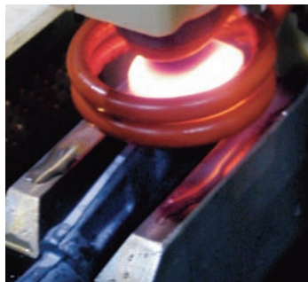
Fig. 1 — Examples of induction hardening; induction surface hardening of camshaft lobes (top), induction through hardening of carbon steel pins (middle), and selective induction hardening of the head of the hammer (bottom).
