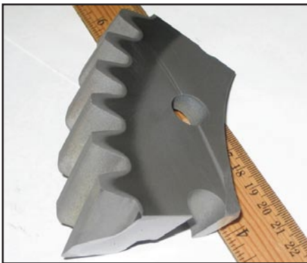
Fig. 4: Induction harden pattern (zoomed) of large helical gear shown in fig. 3.
