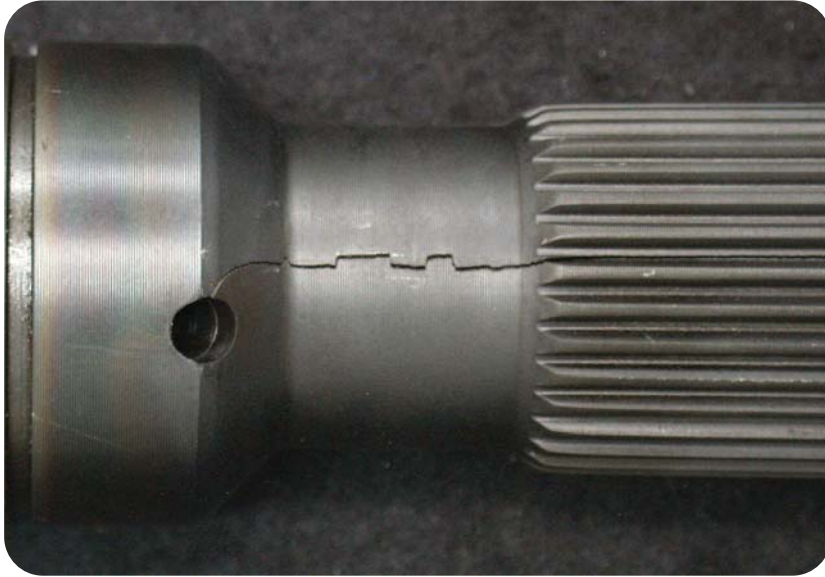
Fig. 5 — Cracking of the hole located at the change in shaft diameter.
