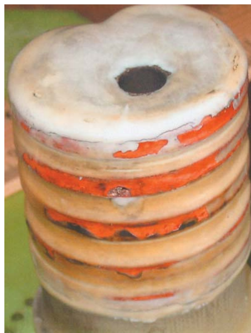
Fig. 3 — Evidence of coil abuse due to improper part/coil handling when inductor can accidentally touch the part.
