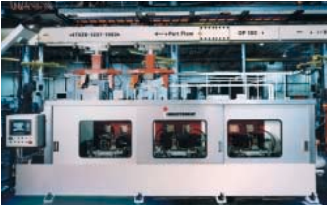
Fig. 3 Photograph of the non-rotational (SHarp-C) crankshaft induction hardening unit.
