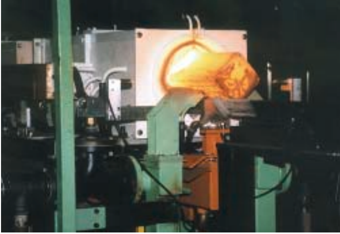
Fig. 4 Rectangular bar exiting and in-line induction bar heater.
