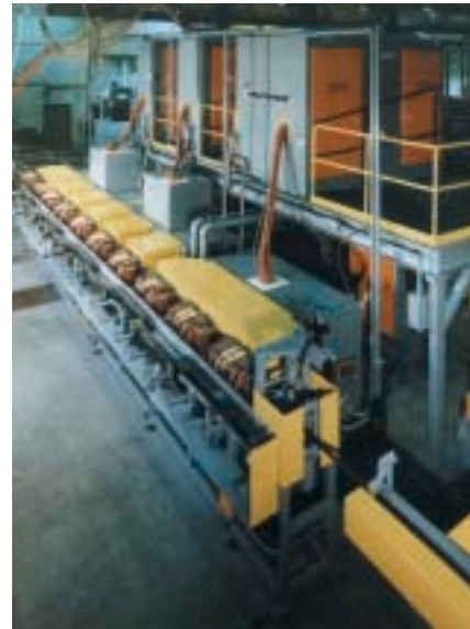
Fig. 3 An induction bar heating line.
