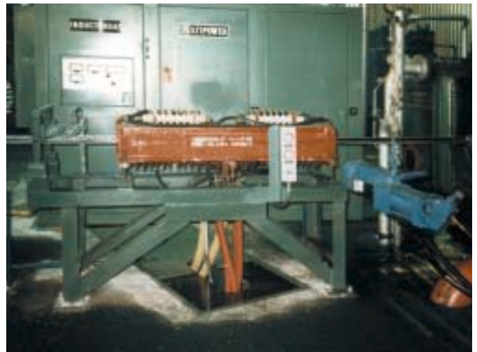
Fig. 6 A compact, medium frequency bar heater improved efficiency and heating quality for an aluminum bar manufacturer.
