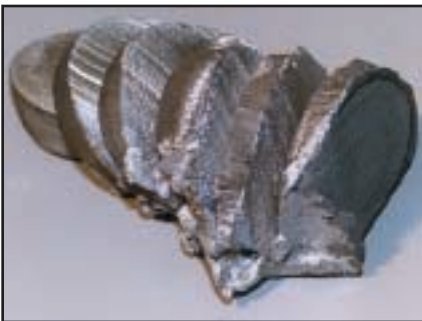
Fig. 1 Sliced aluminum slug in the semi-solid stage.
