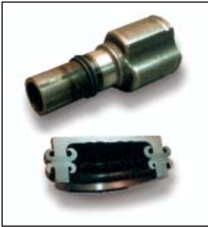
Fig. 2 Friction welded (edge-to-edge induction welded) CV joint and its enlarged cross-section.
