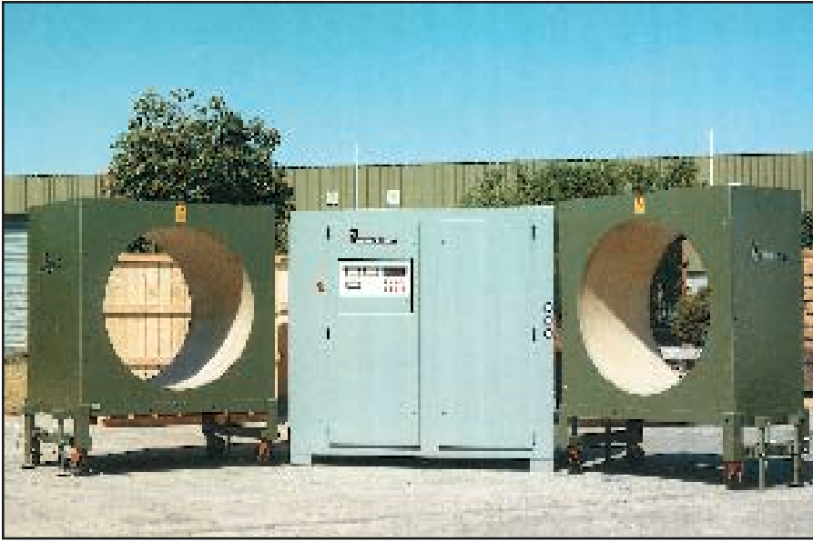
Fig. 8 Induction heating system for pipe coating.
