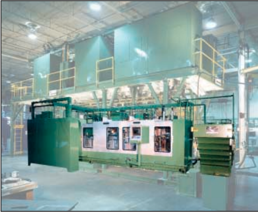
Fig. 2 CV joint heat treating system with heat station power supplies superimposed over a similar system with balcony mounted SCR power supplies.
