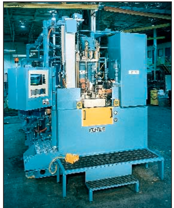
Fig. 3 Cell for hardening camshafts with two heat station power supplies.
