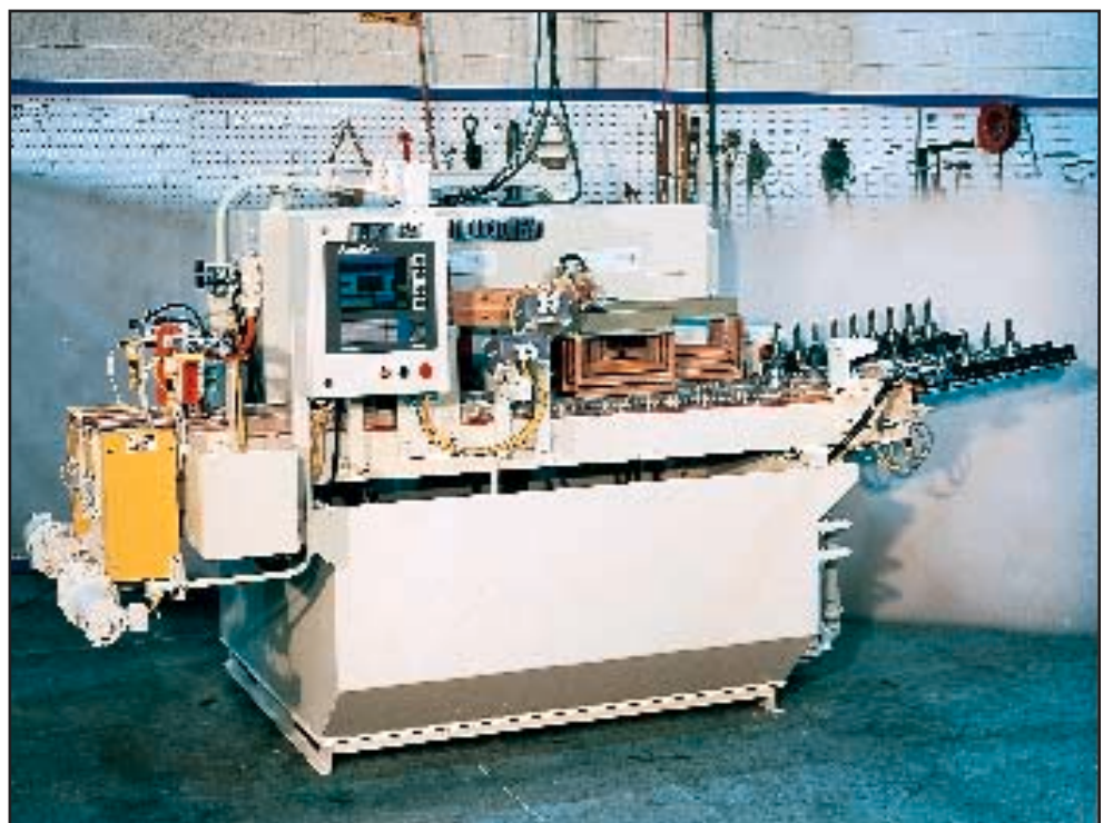
Fig. 5 Compact in-line induction tempering machine.
