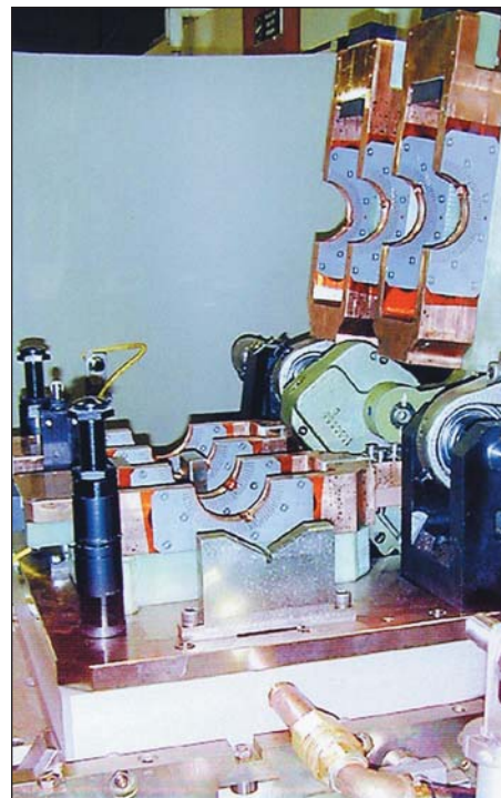
Fig. 4 — SHarP-C coils in the open position. Top coils are passive; bottom coils, active. Ref. 2.
