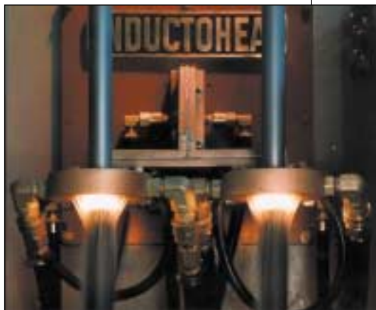
Fig. 1 — A dual-shaft vertical induction scan hardening machine in action. Quenching is taking place below the single-turn MIQ (machined integral quench) inductors.
