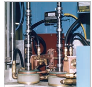
Low distortion camshaft hardening with 25kHz power
