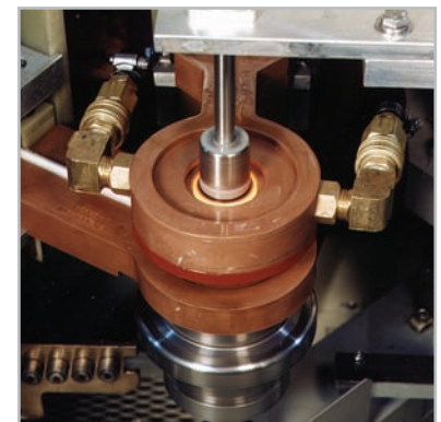
Hardening and tempering a spline
