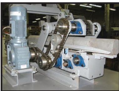
Close-up of heavy-duty twin chain tractor infeed drive
